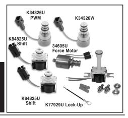
Both A and B shift solenoids are the same. The PWM & the 3-2 PWM are also the same
