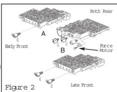
connector to the harness plug and then pull the outer cover connector over it until it clicks into the harness plug on the shift and PWM solenoids. Slide the spade ends into the harness plug with the plug latch sliding across the bridge turned away from the latch on the EPC solenoid. The lock up solenoid located in the pump is the only solenoid with a diode, which has to be wired for proper polarity; positive to positive & negative to negative.
